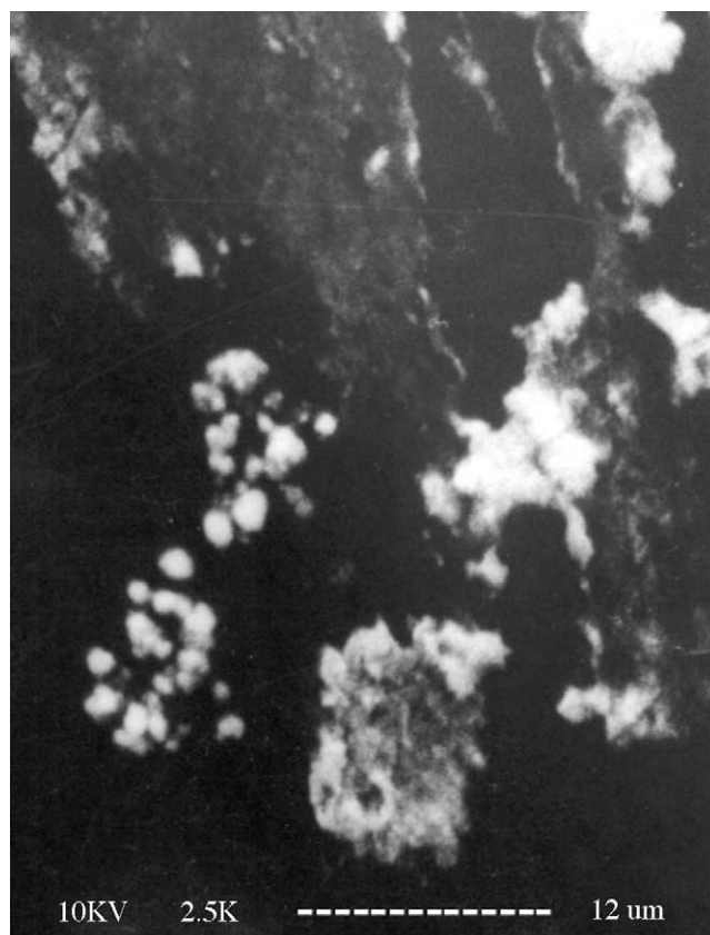
Fig. 1. Scanning electron micrograph of silver nano-particles in water generated by electro-chemical method.
